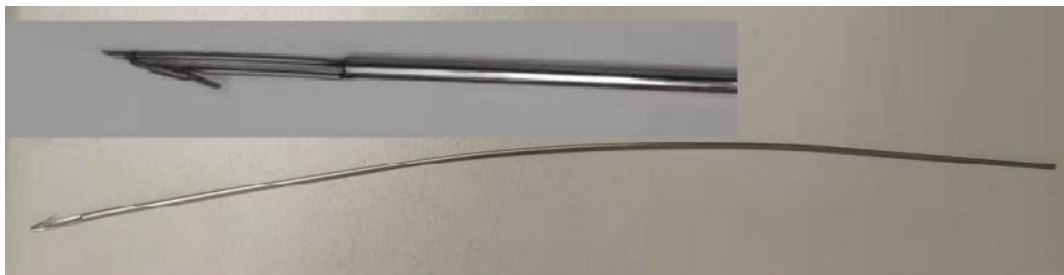
Fig. 2: Appearance of self-made broken nail extractor.
