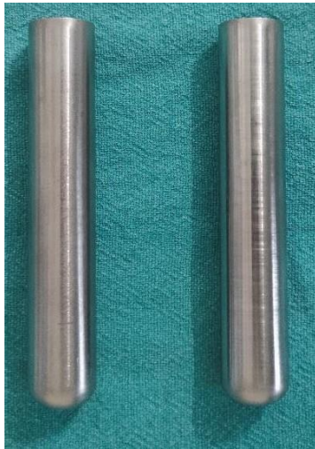
Figure 5 (Titanium test tubes) Figure 6 (Length: 12.5 cm)
