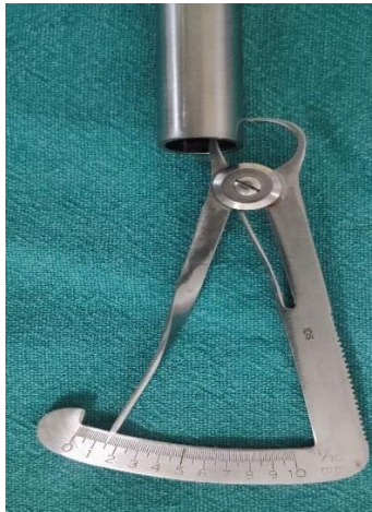
Figure 7 (Diameter 10mm/1cm) Figure 8 (Thickness 1.5mm)
