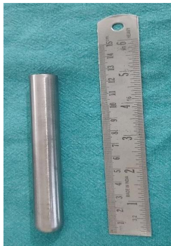
Figure 5 (Titanium test tubes) Figure 6 (Length: 12.5 cm)
