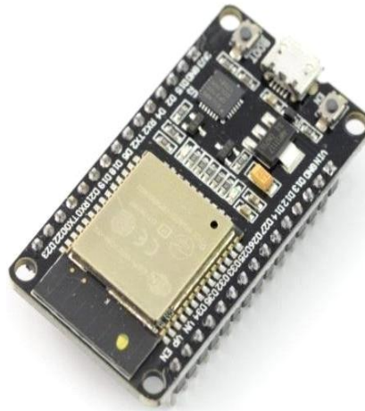
Figure 1.1 ESP32 (Wi-Fi Module) microcontroller chip
