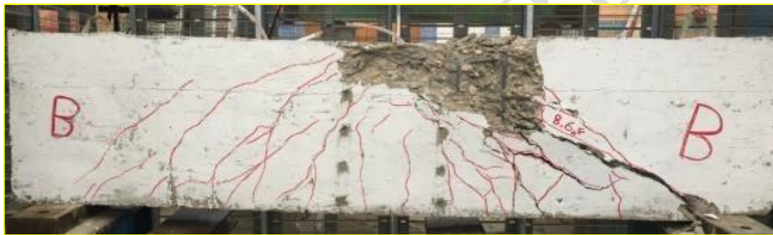
Figure 5. Cracks pattern for experimental tested specimen B at failure.
