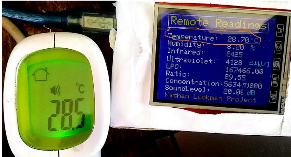
Figure 4: Temperature reading of Infra-red thermometer compared with designed EC-DAQS.
