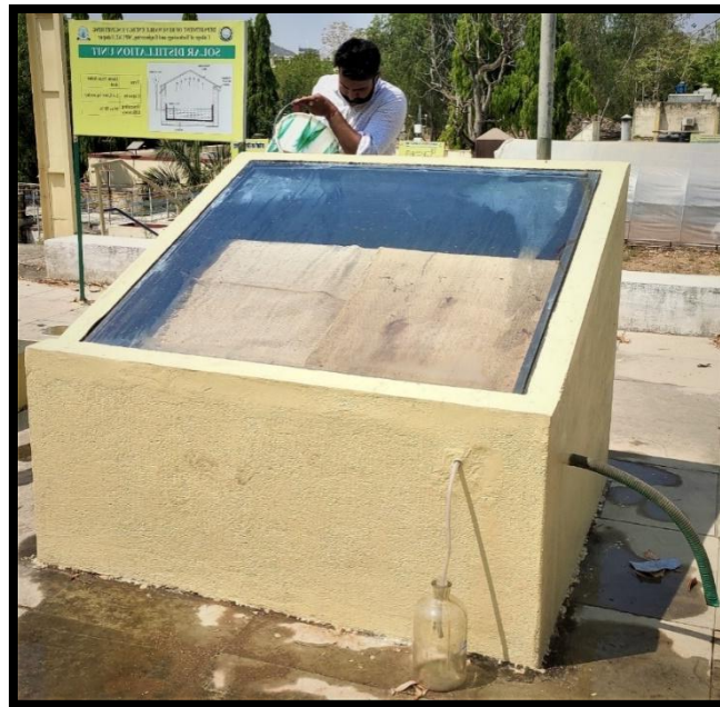
Fig.1 Developed Passive solar distillation unit
