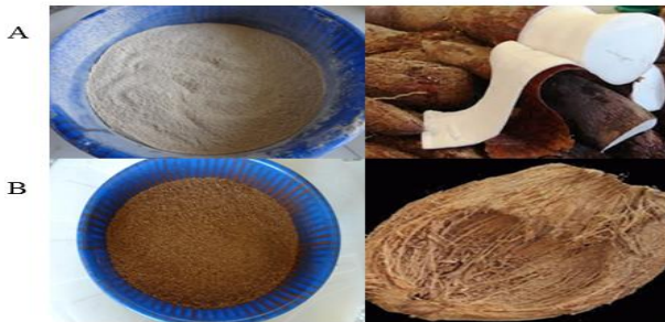
Figure 2. Agricultural waste materials for super absorbent polymer production. A: Cassava mesocarp powder obtained from cassava mesocarp B: Coconut coir dust obtained from coconut husk
