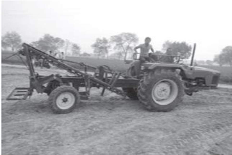
Fig. 3: Tractor mounted carrot digger developed by Naresh
