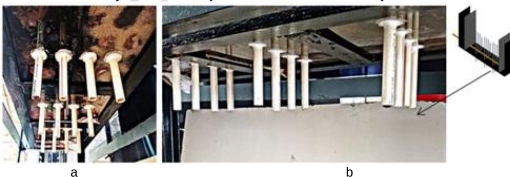
Fig. 12(a), 12(b) Sampling pipes at the bottom of laboratory scale constructed wetland system
