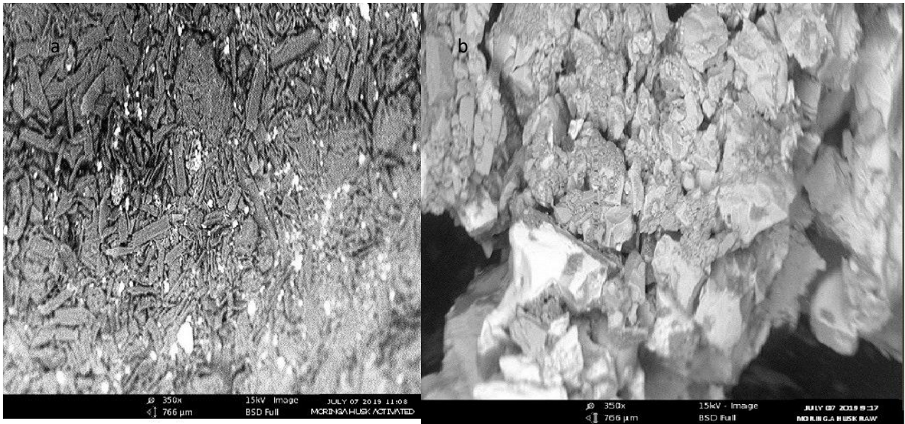
Plate 1: Image of Scanning Electron Microscope of (a) Pure Moringa husk (b) Activated Moringa husks
