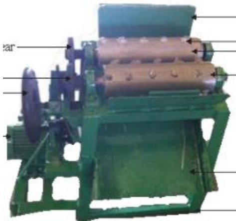
Fig. 1.16 Coconut dehusking machine with flywheel
