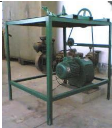
Fig. 1.4 Cam and follower type coconut dehusker
