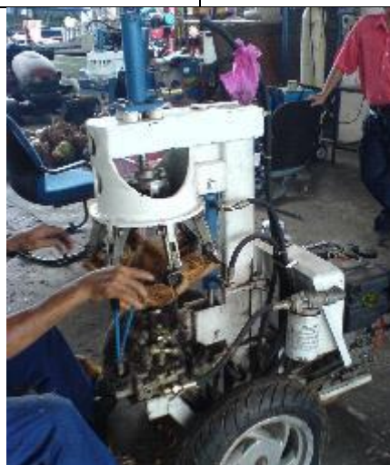
Fig. 1.22 Coconut dehusking machine (model:COM11)
