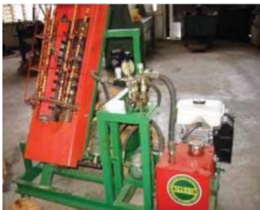
Fig. 1.10 Petrol engine powered coconut dehusking machine
