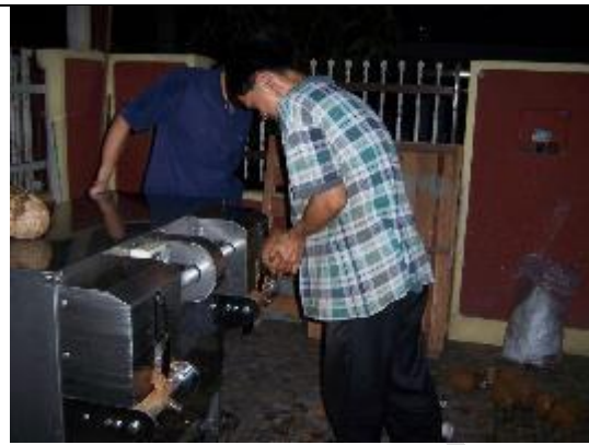
Fig. 2.6 Coconut deshelling machine (Model:COM20)
