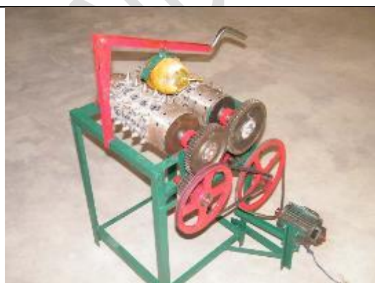
Fig. 1.5 Coconut dehusking machine (Two spiked rolls)
