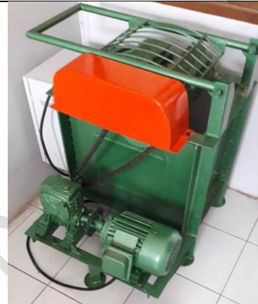
Fig. 1.17 Coconut dehusker machine for small scale industry
