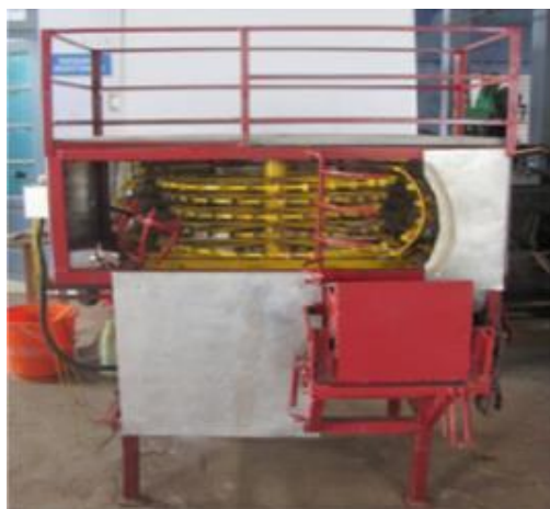
Fig. 1.9 Continuous power operated coconut husking machine with its husk loosening mechanism(a) and husk removing mechanism (b).
