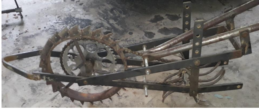
Fig. 5 A view of newly developed rotary weeder
