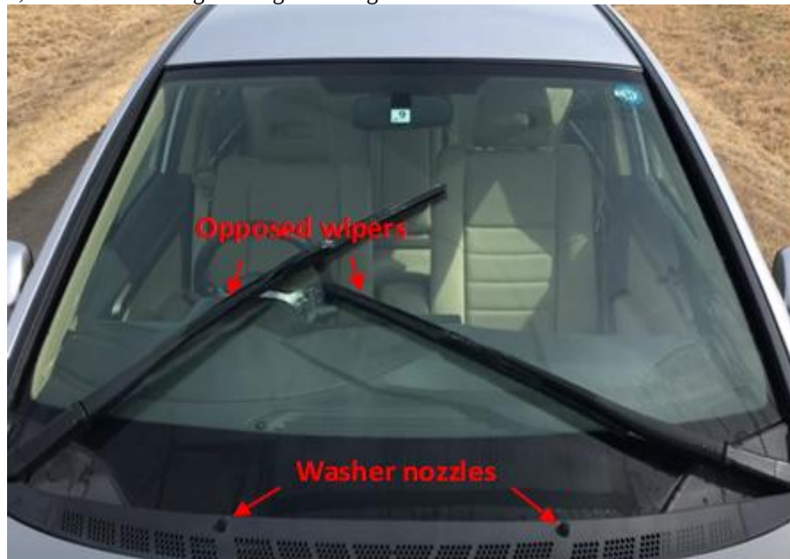
Fig. 16. Opposed pattern wiper blade of Honda Civic [16]
