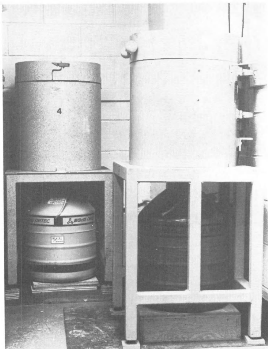
FIG. 3. Germanium detector shields with liquid nitrogen Dewars for cooling.
