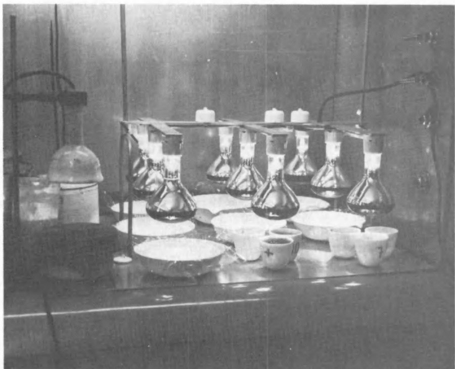
FIG. 7. Evaporation lamps for drying samples.
