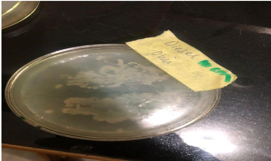
Plate 2: Organisms growing on Minimal Salt Medium supplemented with Diesel as the carbon source.
