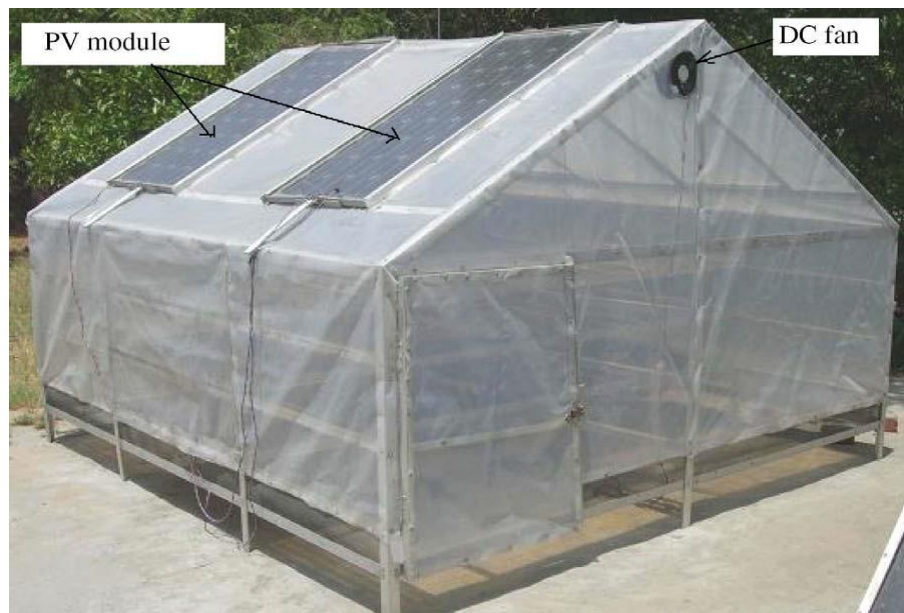
Figure 10: Hybrid photovoltaic-thermal (PV/T) integrated greenhouse dryer
