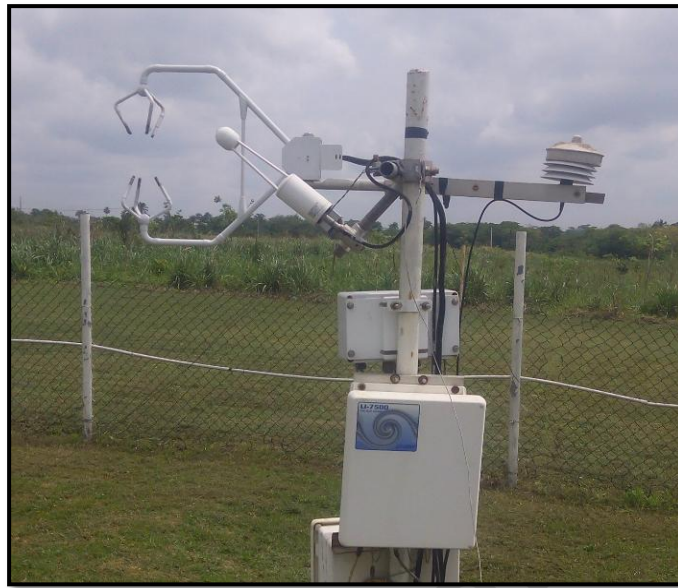
Fig. 1: The Eddy Covariance System deployed at the Study Location
