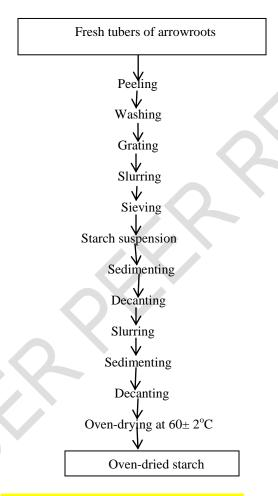
Flow chart for production of arrowroot starch Source: Modified Okereke *et al.*, (2021)
