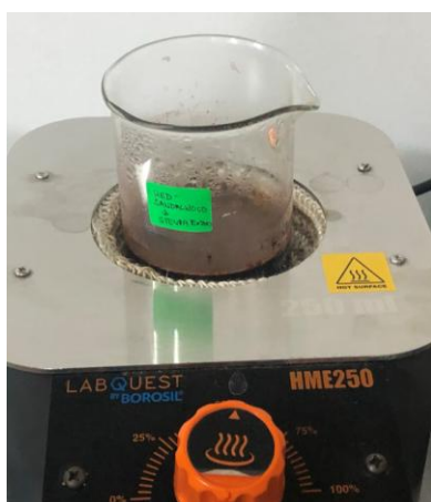
Figure 2: Heating Pterocarpus santalinus and Stevia extract at 70°C for 10 minutes for the preparation of plant extract.
