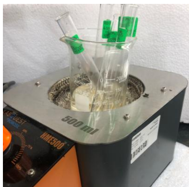
Figure 4: Antidiabetic activity was performed by adding DNSA reagent to stop the reaction and the solution was heated in a water bath for 5 minutes.
