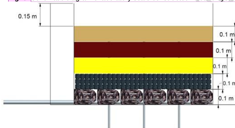
Fig. 6. Thickness of the each layer in laboratory scale constructed wetland system
