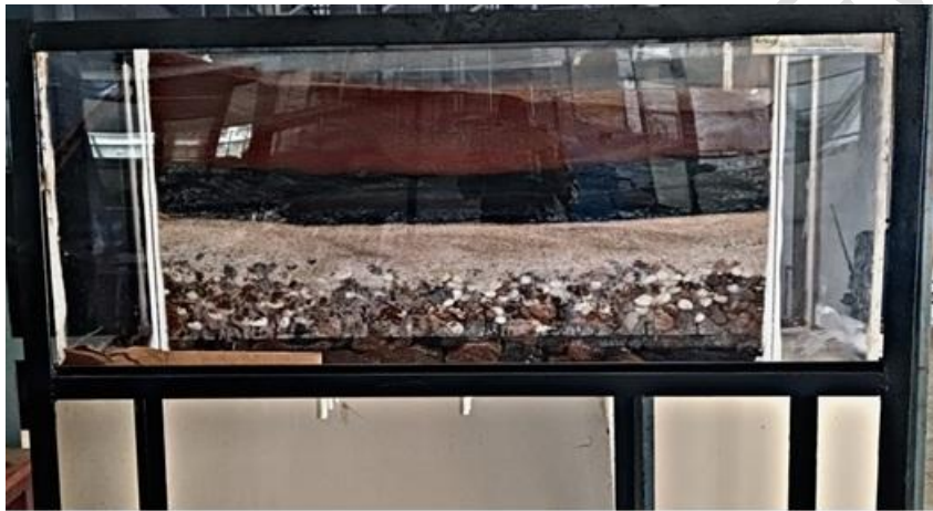
Fig. 10. Constructed wetland in laboratory scale after arranging the media
