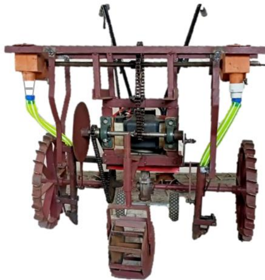
Figure.5 Prototype two row maize dibbler
