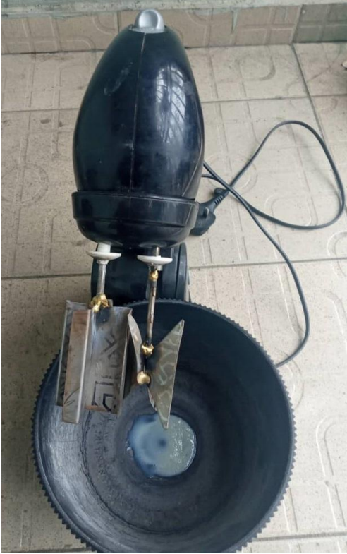
Plate 3. Mixing the Slurry with the Two Z - TETE Blades Hybrid Stirrer Arm.
