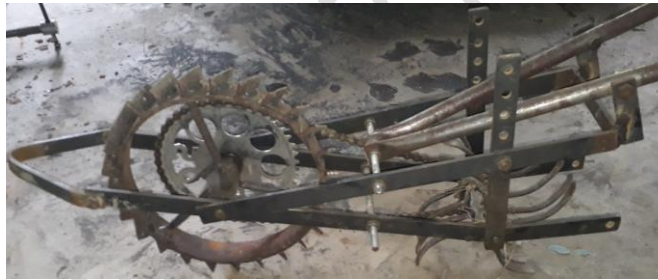
Fig. 5 A view of newly developed rotary weeder
