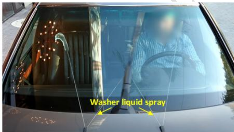
Fig. 10. Washer nozzle function of Mercedes-Benz W124 [11]
