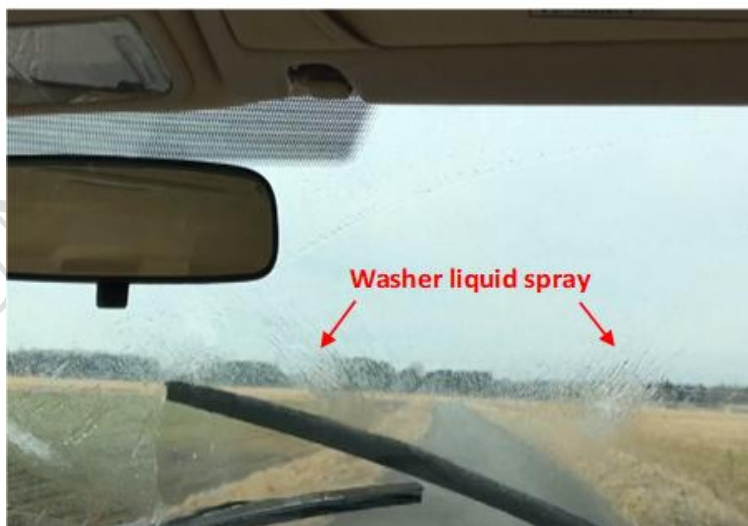
Fig. 17. Spray of washer liquid on Honda Civic [16]
