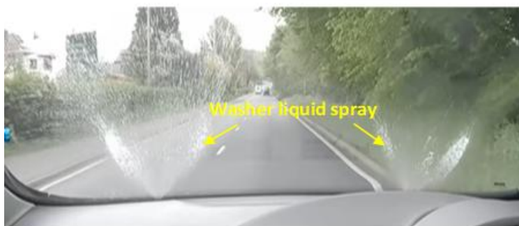
Fig. 15. Spray of washer liquid on SEAT Altea [15]
