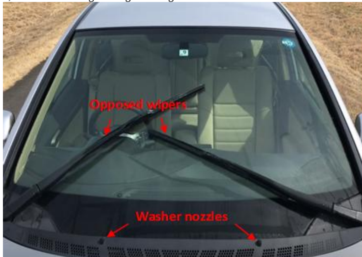
Fig. 16. Opposed pattern wiper blade of Honda Civic [16]
