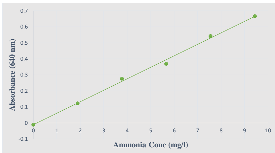
Figure 3. Standard curve of ( \text{NH}_3 , \text{NH}_4^+ ) and correlation equation Y = -0.0112 + (0.0717)X where Y is Absorbance, and X is Ammonia concentration (mg/l). This equation permits to calculate ammonia concentrations in the mini-pond during experimental time.
