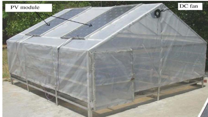
Figure 10: Hybrid photovoltaic-thermal (PV/T) integrated greenhouse dryer
