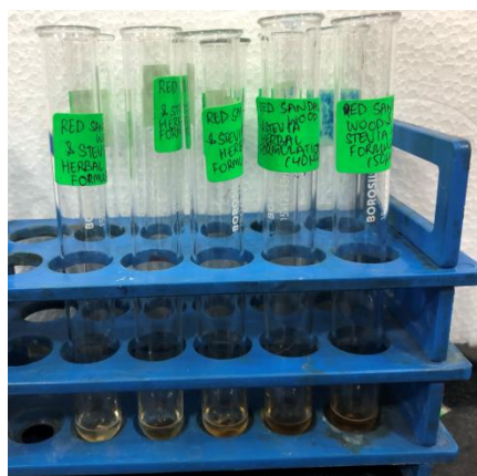
Figure 3:Antioxidant activity performed by adding 1ml of DPPH in methanol and then the reduction in the quantity of DPPH free radicals was assessed dependent on the absorbance at 517nm.
