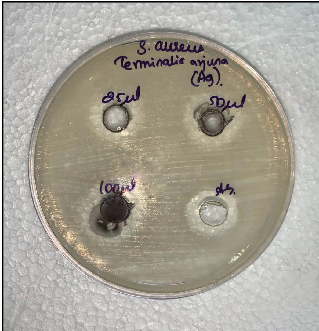
Figure 4 - Showcasing the effect of various concentrations of Ag-NPs on Staphylococcus aureus with their zones of inhibition:
