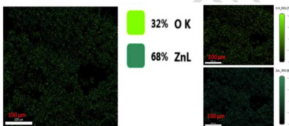
Figure 6: Elemental Mapping analysis of synthesized ZnONPs
