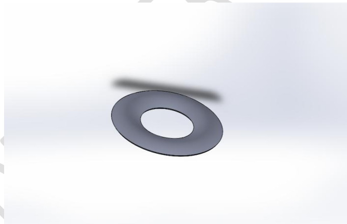
Figure 2: SolidWorks 2014 illustration of Concave Rigid-ring Baffle with pitch of 0.0200 m
