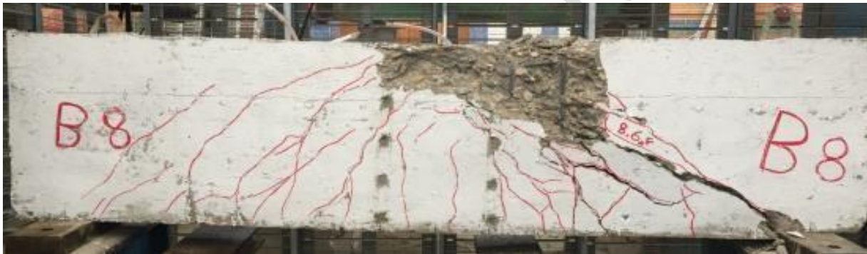
Figure 5. Cracks pattern for specimen B8 at failure.
