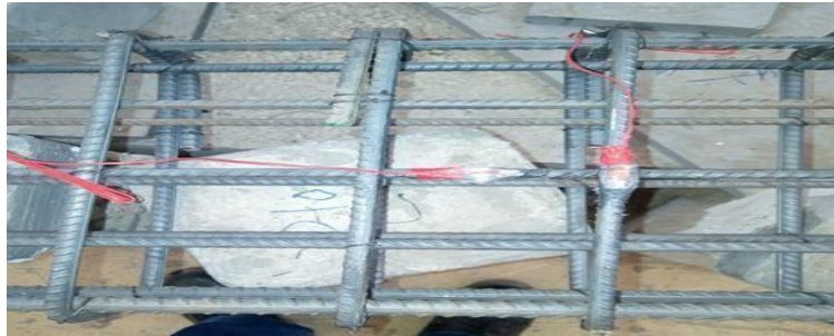
Figure 3. Installation of strain gauges.
