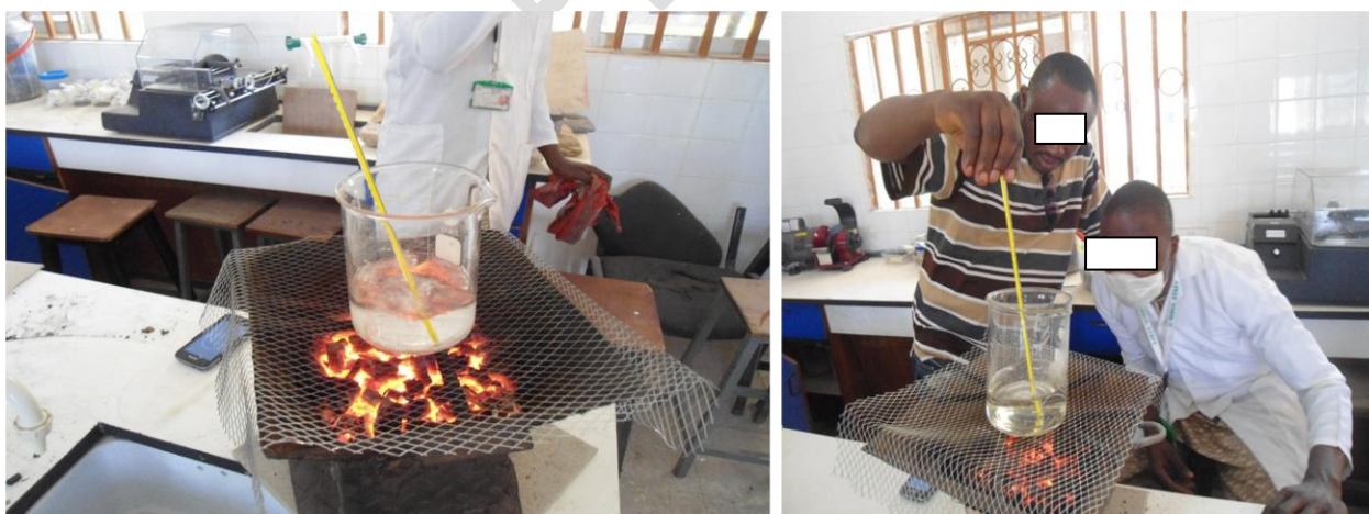
Fig. 8. Combustibility studies for the determination of the coal energy efficiencies and coal combustion pathways by measuring the time it takes same quantity of each of the coal deposits to bring same volume of water to boiling point as well as the temperature achieved at every 2 minutes using local cooking stove
