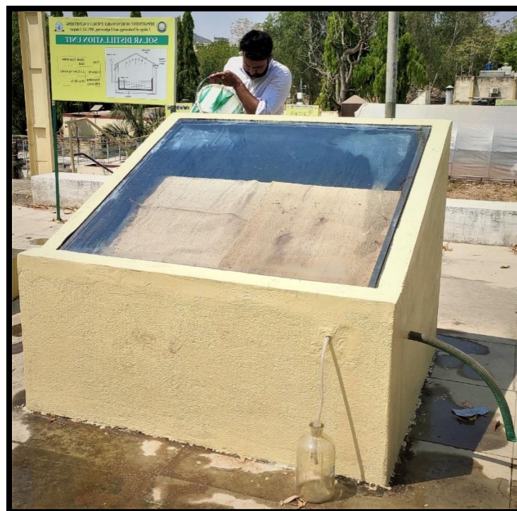
Fig.1 Developed Passive solar distillation unit
