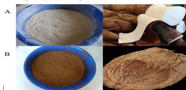
Figure 2. Preparation of organic waste materials: (A) Cassava mesocarp powder and (B) Coconut coir dust.
