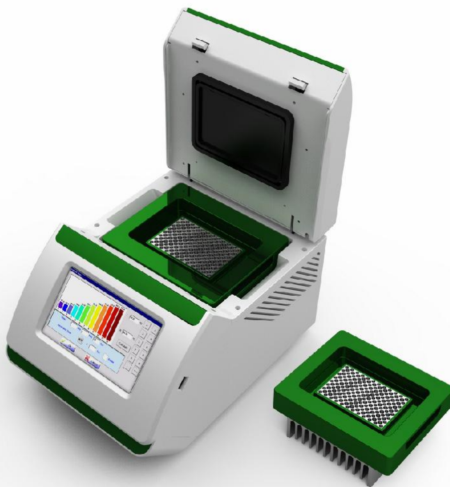
Figure 1- Diagram showing a Polymerase Chain Reaction Machine (Thermal Cycler) [3]
