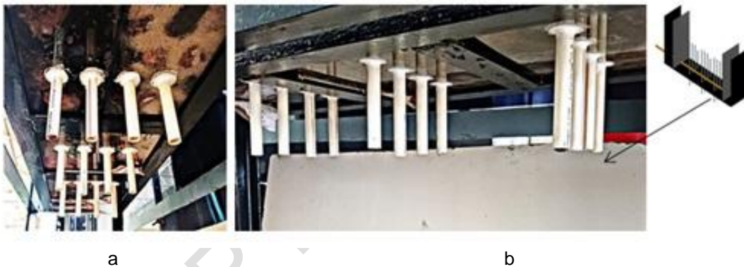
Fig. 14(a), 14(b) Sampling pipes at the bottom of laboratory scale constructed wetland system
