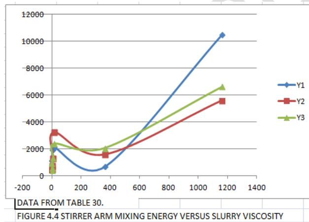
**Figure 4: Stirrer Arm Mixing Energy Versus Slurry Viscosity.**
