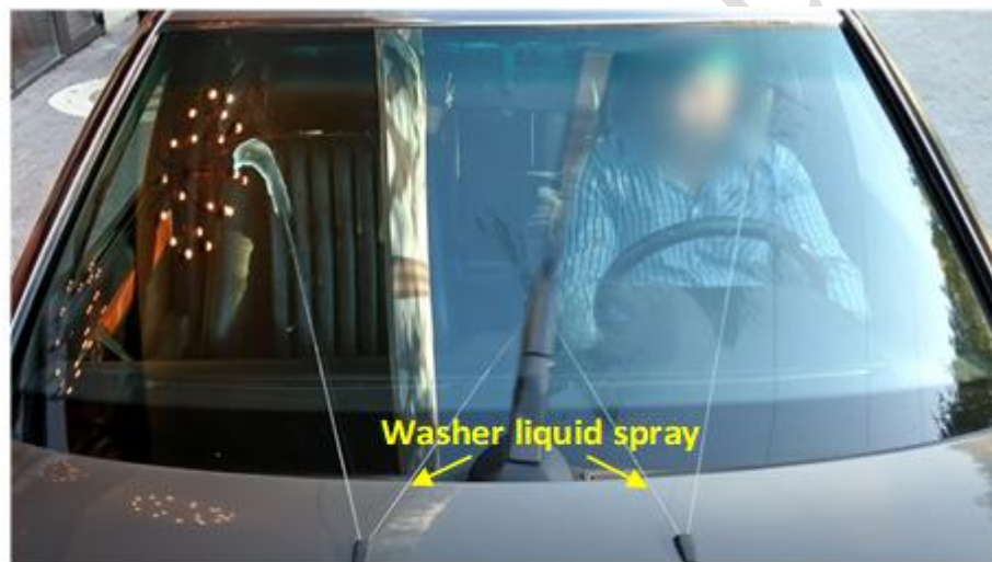
Fig. 10. Washer nozzle function of Mercedes-Benz W124 [11]
