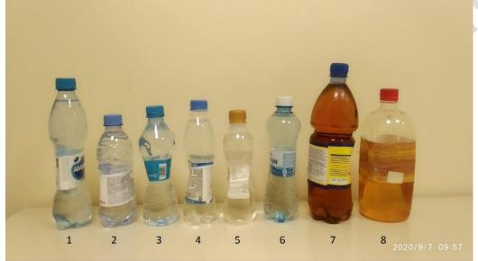
Attributes: The #1-4 and #6 bottles are non-carbonated drinking water from various manufacturers; #5 bottle is chemical solvent "646"; #7 bottle is drying oil; and #8 bottle is alkyd varnish (the bottle was initially incomplete). The bottles were evaluated at a temperature of 24
