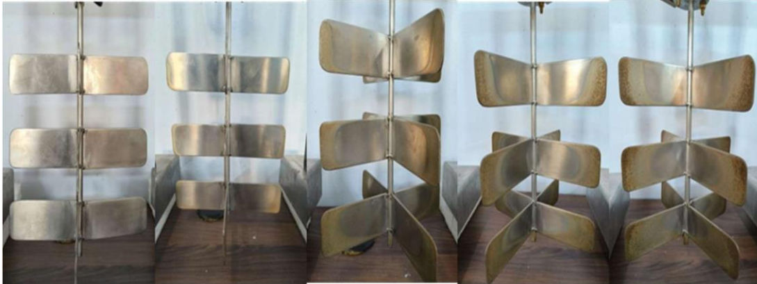
Figure 10: Effect on the surface of the agitator after ohmic heating of milk
