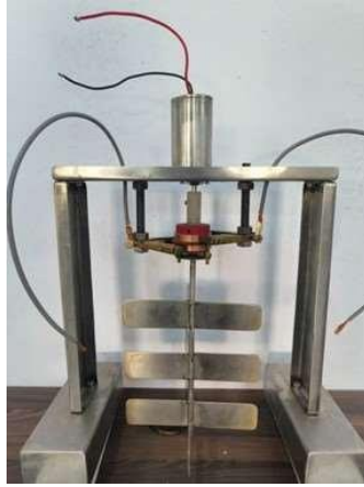
Figure 2: Agitator, motor and slip ring assembly
