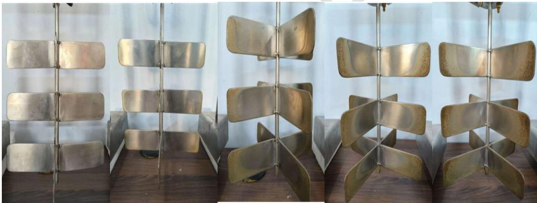
Figure 6: Effect on the surface of the agitator after ohmic heating of milk
