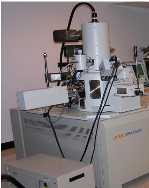
Figure 2: Scanning Electron Microscope Model JOEL-JSM 76000F
