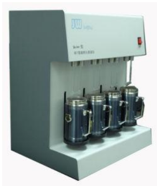
Figure 1: BET Surface Area Analyzer Model No JW-DA: 76502057en
