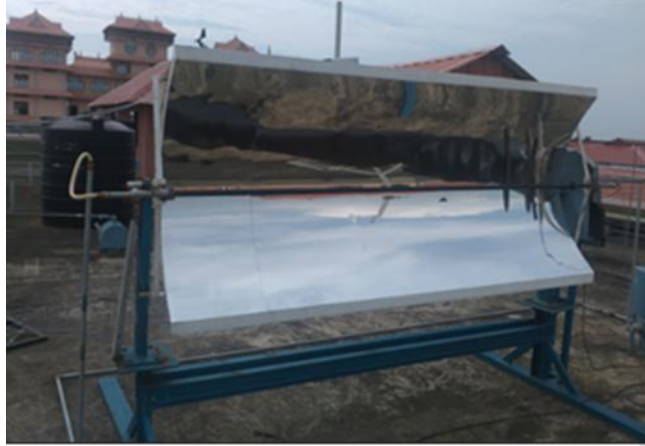
Fig.3 Experiment setup using stainless steel tube as receiver tube
