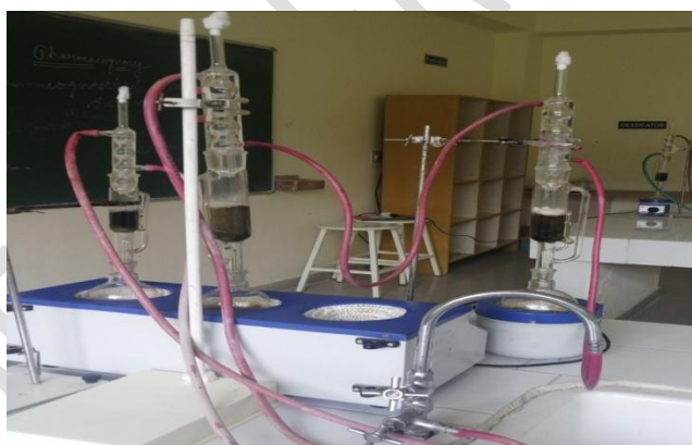
Fig.2. Soxhlet assembly for extraction
