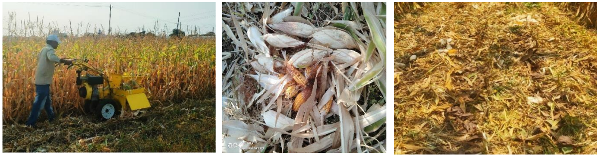
Fig. 2: Field testing by the machine, total cobs obtained and residue management after harvesting
