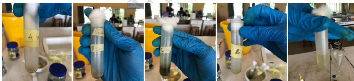
Fig 3. Separation of organic from aqueous phase in mixture after addition of chloroform:isoamyl alcohol using separatory funnel
