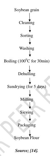
Figure 2. Flow chart for the processing of Soybean into Flour.
