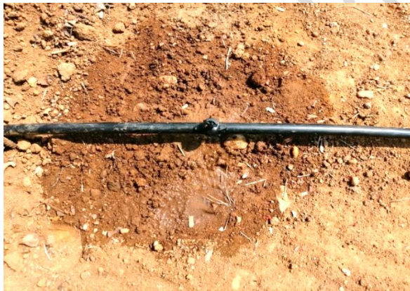
Fig. 3 Horizontal water zone radius of 4 lph dripper
