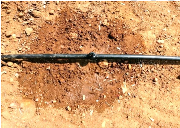
Fig. 3 Horizontal water zone radius of 4 lph dripper
