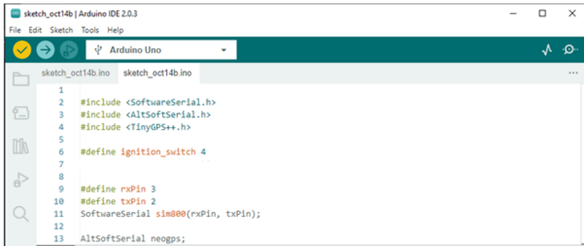
Figure 12: Library and serial communication setup
